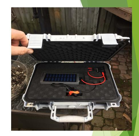
Solar-powered by 6 watt panel and "Always On" capable battery pack
